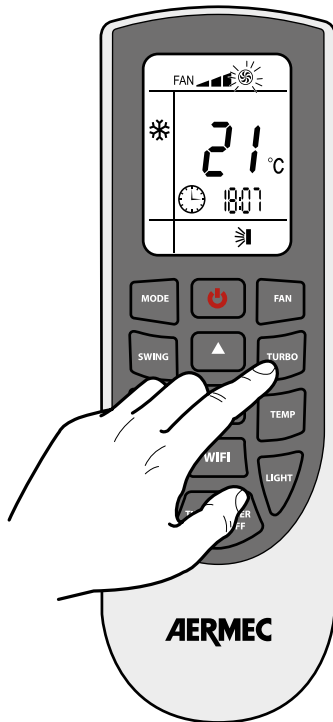
Setting the TURBO function
