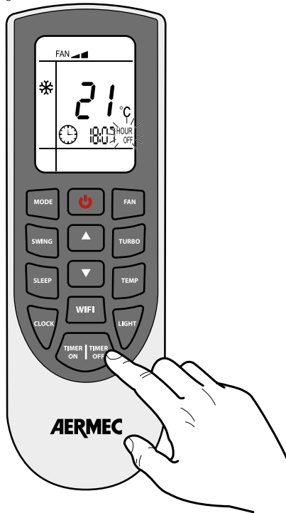
Setting a programmed deactivation
