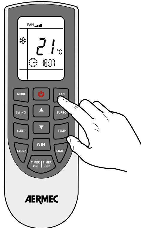
Setting the ventilation speed
