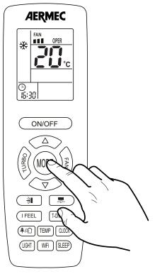
If the unit is on, pressing the work button allows passing from one operating mode to the next, in this sequence:
