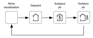
NOTE: The default display on the indoor unit's display is the operating setpoint; the room temperature value is displayed for 3 seconds after which the display returns to the operating setpoint. To display the room temperature again it is necessary to select the corresponding symbol on the remote control.
