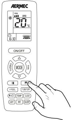
If the unit is on, while pressing the button it activates the swing of the motorized supply air fin. The fin allows to change the air flow in the room depending on the set position; When the unit is on, while pressing the button it's possible to set one by one the following steps:
