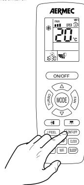
NOTE: Once a programmed switch on is set, the operating mode, the working setpoint and fan speed, will be the same as those present when the unit stops.
