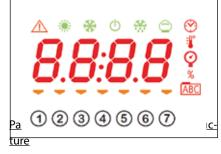
Parameters on the device can be changed from the keyboard. Access to the various parameters is organised in sub-levels, which can be accessed by pressing at the same time the keys "esc" and "set" (see above). Each menu level is identified by a mnemonic code that can be seen on the display. For further information, see the following page.
