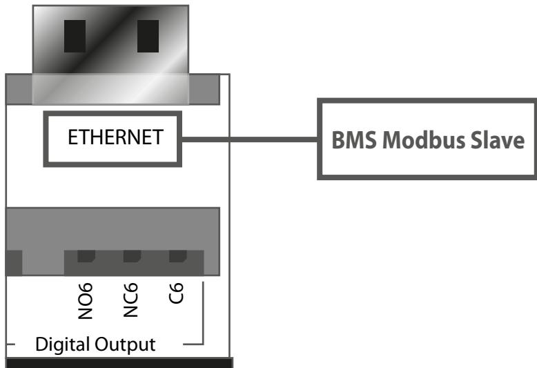
The BMS communication cable must be connected to the Ethernet port identified on the figure as "BMS Modbus Slave"
