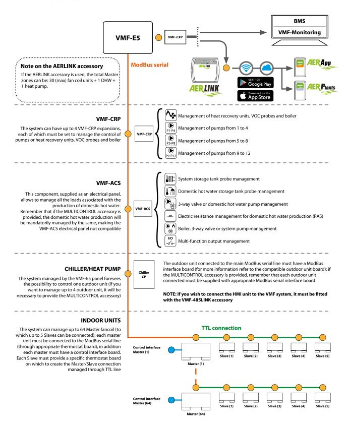
**ATTENTION:** if one (or more) areas are controlled with an FCWI fan coil (each of which require the VMF-485LINK interface), these areas cannot have a Slave unit.
