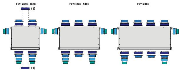
1 There is a central preparation for the installation of an accessory BRY220 as an alternative to using the two more external preparations.
