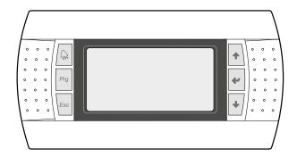
The command panel of the unit allows the rapid setting of the working parameters of the machine, and their visualisation. The card stores all the default settings and any modifications.
