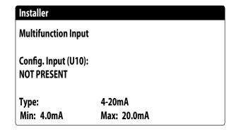
**U10**: this value indicates which function to assign to the multifunction input U10; the possible states are:
