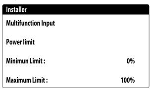
**Minimum limit**: this value indicates the minimum power level that can be reached based on the input signal;
