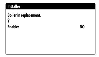
**Boiler enabled as replacement**: this parameter indicates whether to activate the boiler if the outside temperature drops down below the "replacement" value specified in the following window, or if the heat pump has a "total alarm";
