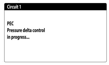
If the result of the pressure delta control is greater than 15 bar (and the 4-way must switch), the valves must be controlled without the activation of the compressors to reduce the pressure delta; Alarms (warnings) are not generated in this situation). If the control is less than 3 bar (hot/cold operation or a 4-way must switch), the compressors are started without the valve control in order to create the pressure delta; after 300s in this situation an alarm is generated with a machine block.
