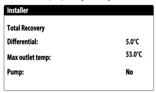
**Differential**: indicates the differential used in the adjustment to calculate the power necessary for recovery;
