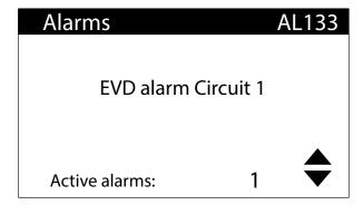
By pressing the list of active alarms is displayed. Each alarm is uniquely identified by a 4-digit alarm code, this code can be found on the previous pages.
