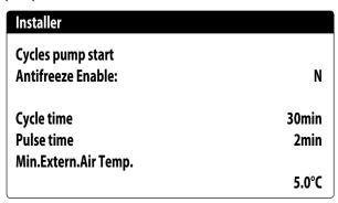
**Enable pump cyclical start-up for anti-freeze**: this value indicates whether to enable the pump start-up cycle for the anti-freeze function;
