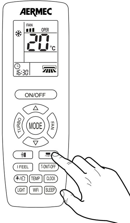
If the unit is on, while pressing the button it activates the swing of the motorised supply air fin. The fin allows to change the air flow in the room depending on the set position; When the unit is on, while pressing the button it's possible to set one by one the following steps:
