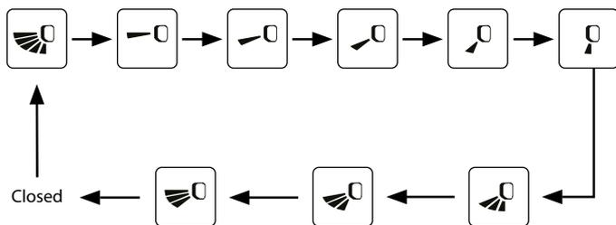
**Note:** operate continuously up & down swing in 2 seconds, swing states will change according to above-mentioned order, or switch closed state and "state."
