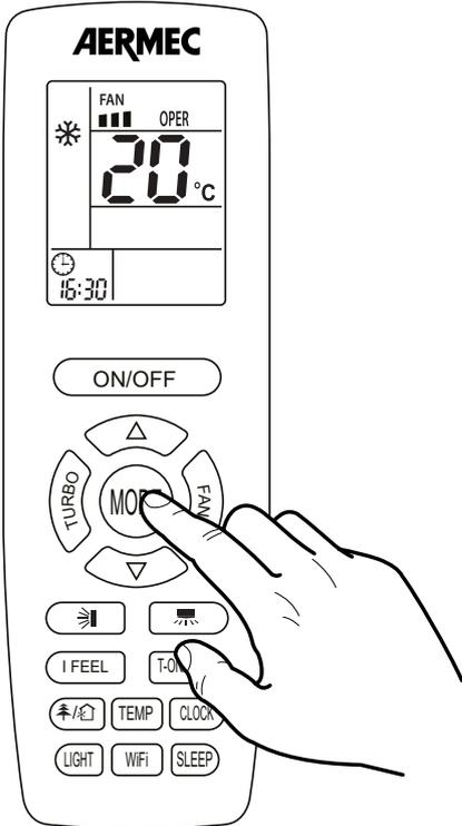
If the unit is on, pressing the
