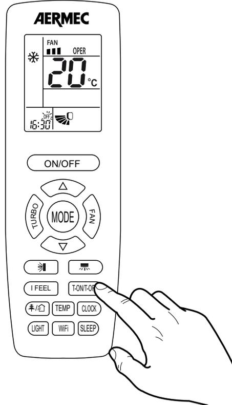
**NOTE:** Once a programmed switch on is set, the operating mode, the working set-point and fan speed, will be the same as those present when the unit stops.
