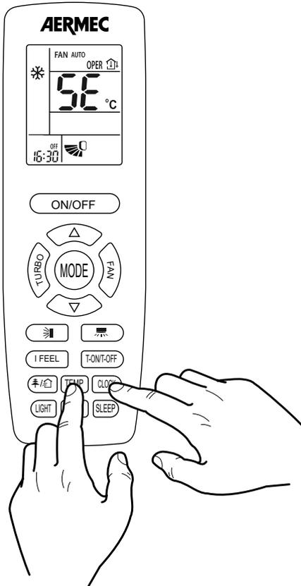
**NOTE:** The energy saving and night-time functions can not be activated at the same time; if the night-time wellness function is active and you want to activate the energy-saving function, the night-time wellness function will be disabled automatically. Under energy-saving function, fan speed is defaulted at auto speed and set temperature and speed can't be adjusted. Press "TURBO" button and the remote controller won't send signal.
