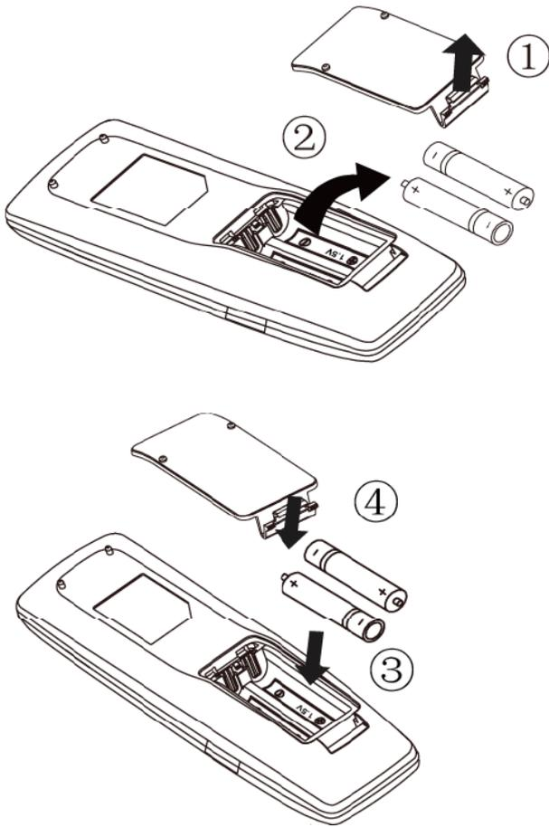
To replace the batteries of the infra red remote control proceed as follows:
