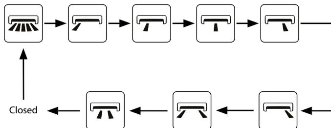
**Note:** operate continuously left & right swing in 2 seconds, swing states will change according to above-mentioned order, or switch closed state and "state."
