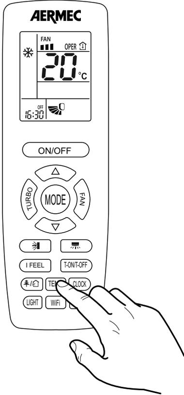
Through the use of the remote control it is possible to display the room temperature value read by the indoor unit, or display the current operating setpoint used by the unit. This information is displayed on board the indoor unit's display. Under on status, receiver light board or wired controller is defaulted to display setting temperature. Press "TEMP" button to view indoor ambient temperature.
