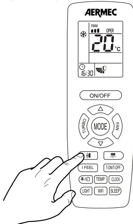
If the unit is on, pressing the button allows the activation of the swing function of the motorised discharge fin. This fin varies the direction of the flow of air into the ambient, on the basis of the selected position; With the unit on, pressing the button allows the setting of the following sequenced steps, one by one:
