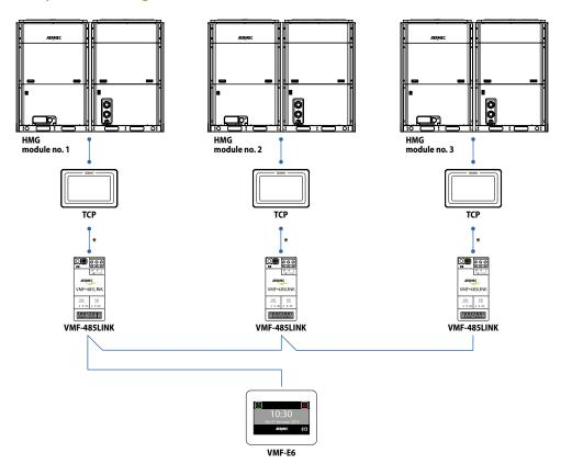
$<sup>\</sup>ensuremath{^{*}}$  Connection to be made with the aid of the accessory IC-2P.
