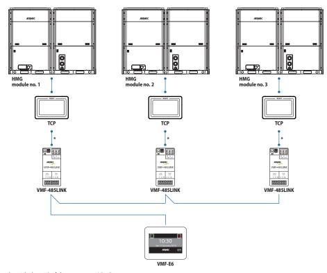
\* Connection to be made with the aid of the accessory IC-2P.
