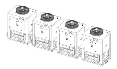
Each machine is supplied with 4 grooved joints and two caps (machine input and output defined by the user depending on where the caps are positioned).
