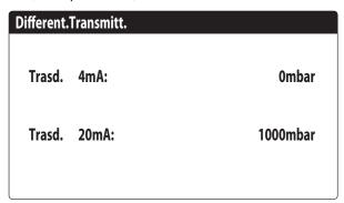
**Transd. 4mA**: minimum limit 4mA **Transd. 20mA**: maximum limit 20mA
