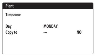
Each program has 8 days and each day has four time periods at which the switch-on and switch-off time, set point 2 or switch-on/switch-off can be set.
