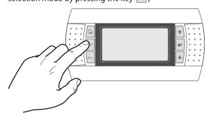
Once in the menu selection mode it is possible to move between menus using the arrow keys: the key to move to the previous menu, and the key to move to the next menu:
