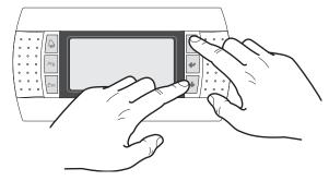
When the desired parameter is seen press the key enter the parameter. To exit the parameter and return to the parameter selection mode press the key.
