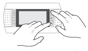
When the desired menu is seen press the key to enter the menu. Press the key to return to the menu selection mode:
