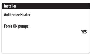
**Pump ON power**: this value indicates whether or not to activate the system pumps during operation of the anti-freeze electric heater;
