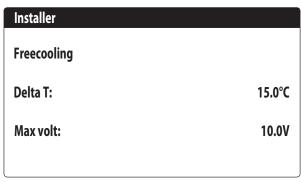
**Delta T**: value generated at the maximum fan speed at a design external air temperature;
