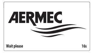
This window indicates the seconds remaining until the software loaded in the unit starts up (switching to the system language selection);
