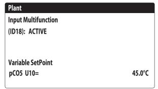
Digital Input ID18: this value indicates the state of the digital input connected to multifunction input (U10) enabling, whose states can be:
