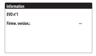
This mask displays information concerning the EVD valve connected in Modbus (if present).
