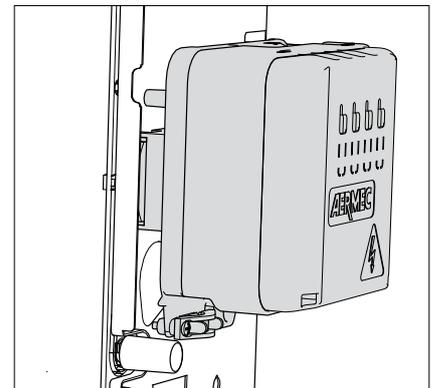
**DANGER:** it is compulsory to tighten the screw on the side of the fan coil, as this is what allows the earth connection of the entire system.
