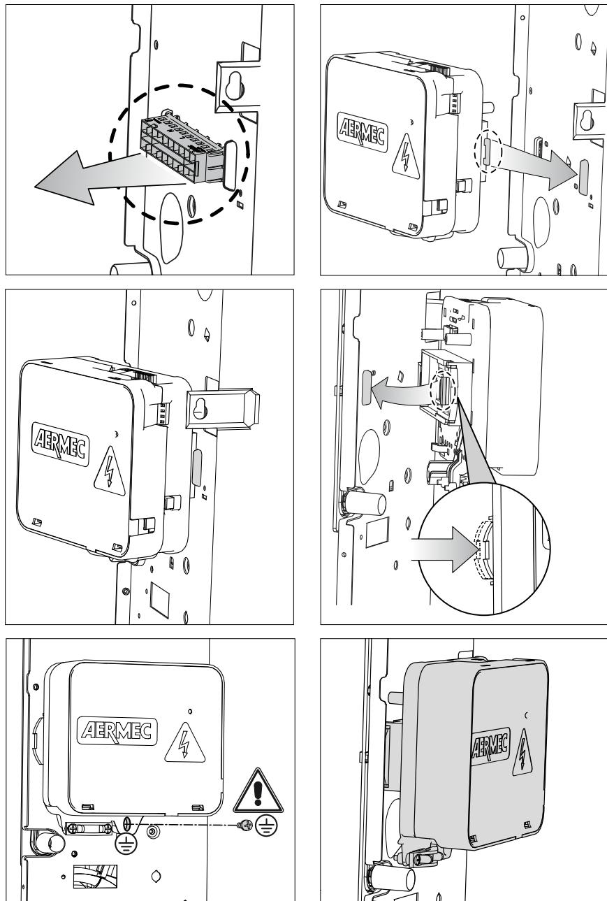
**DANGER:** It is compulsory to tighten the screw that fixes the thermostat box on the side of the fan coil, as this is what allows the earth connection of the entire system.
