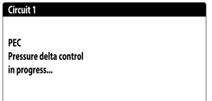
If the result of the pressure delta control is greater than 15 bar (and the 4-way must switch), the valves must be controlled without the activation of the compressors to reduce the pressure delta; Alarms (warnings) are not generated in this situation).
