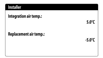
**Integration air temp.**: this value indicates the outside temperature above which the heat pump functions without the aid of the electric heaters, whereas if the outside temperature is lower than this value, but still higher than the replacement temperature, the heat pump functions TOGETHER with the heaters;
