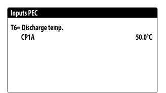
T6: this value represents the temperature of the discharge gas on compressor 1A;
