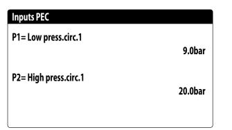
P1: this value represents the low pressure detected by the transducer;
