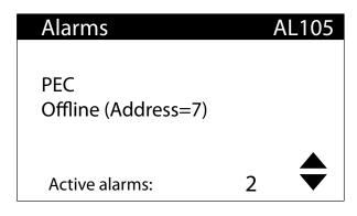
By pressing 🖾 the list of active alarms is displayed. Each alarm is uniquely identified by a 4-digit alarm code, this code can be found on the previous pages.
