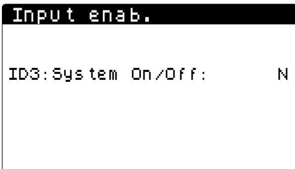
**Enabling ID3:** this value indicates the enabling to use digital input ID3 to manage the remote ON/OFF function (ON = closed / OFF = open).
