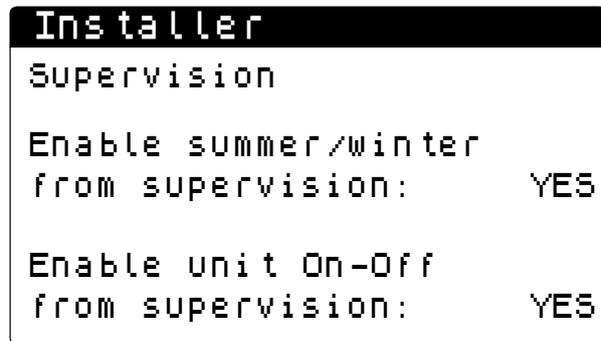
1. **Enable season change from BMS:** this value (not present on WWMG only cold) indicates if the remote season change command for the unit is enabled or not for the unit using the BMS
