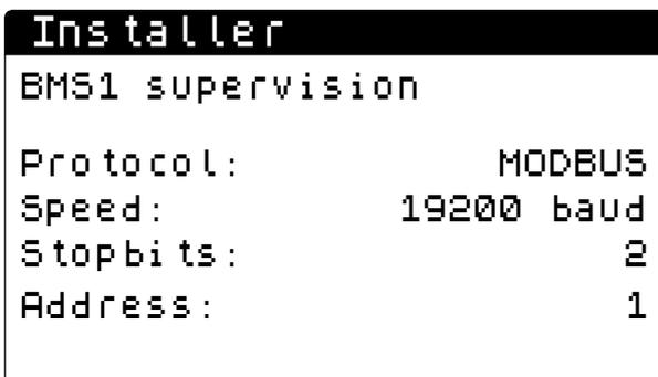
1. **Select protocol:** this value indicates which protocol is used to communicate with the BMS supervision system; the support protocols are:
