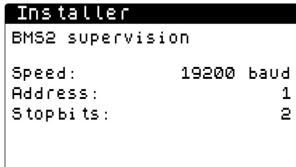
1. **Transmission speed:** this value indicates which speed is set for serial communication
