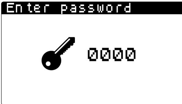
**Menu password:** this value indicates the password to use to access the installer menu; remember that for access, the default value (0000) must be entered.
