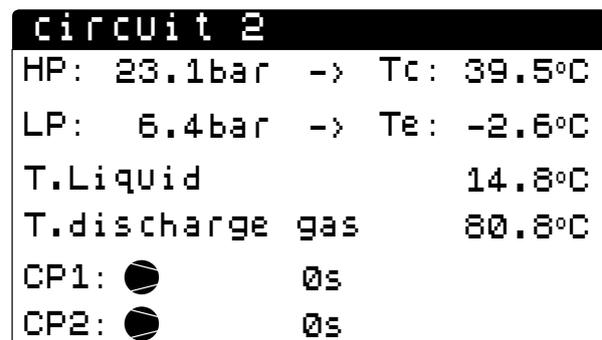
1. **High pressure value:** this value indicates the delivery pressure in the circuit
