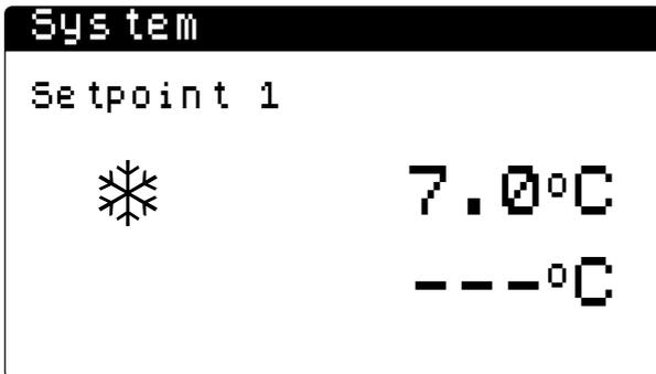
**Main cooling/heating setpoint:** this value indicates the main work setpoints used during the cooling/heating mode.
