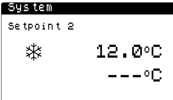
**Secondary cooling/heating setpoint:** this value indicates the secondary work setpoints used during the cooling/heating mode.
