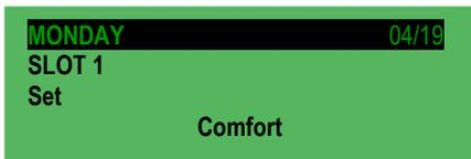
Once the MODE in which the machine must operate in slot 1 has been determined, press the ESC button once to return to the previous menu
