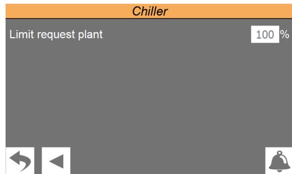
Set a potential power request limit of the thermostat to prevent alarm conditions or set a maximum ceiling on unit consumptions.
