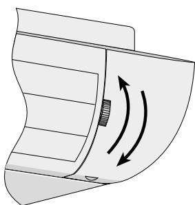
Switching the front air outlet or from the top, using the selector on the unit.
