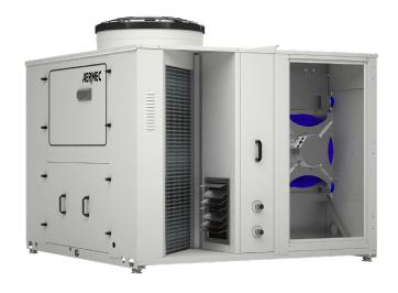
Independent Roof-Top air-cooled air conditioner to treat, filter and renew air based on the selected configuration. Being fitted to function with 30% external and expelled air (MB4 versions), RTX units are designed for medium density applications like shopping malls, shops, offices and production areas.
